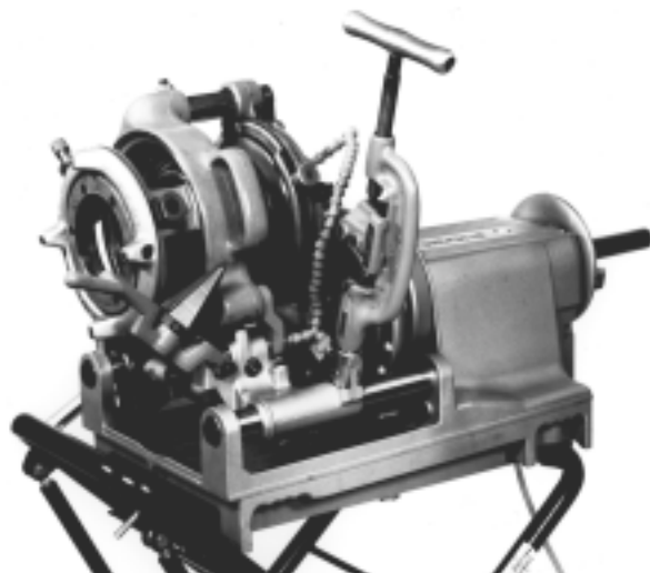
Figure 25 – No. 141 Geared Threader Mounted to 300 Compact
