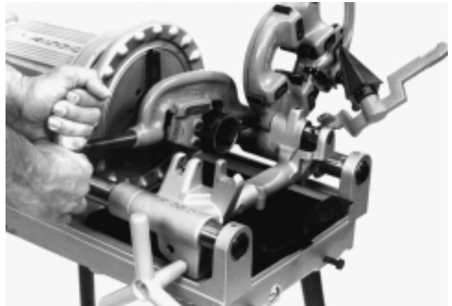
Figure 7 – Cutting Pipe With 300 Compact Threading Machine
